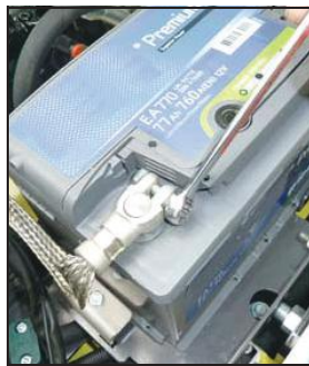
Fig. 10-1 Loosening the terminals
