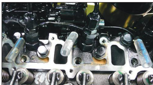
Fig. 10-18 Insulate the connection cable
