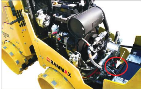
Fig. 9-29 Cable/connector Y9 under the hood
