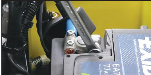
Fig. 10-9 Disconnect the battery
