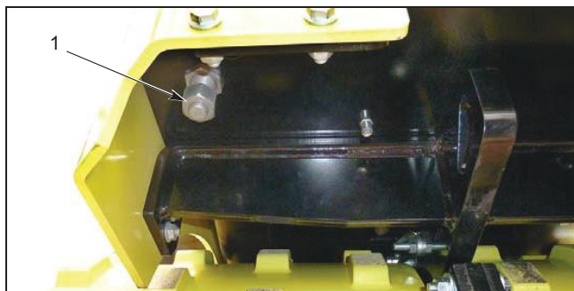
Fig. 9-5 Diesel drain, rear left on chassis
