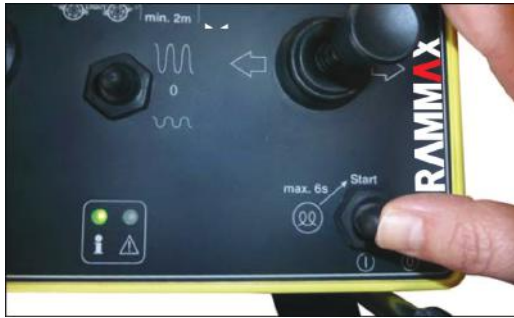
Fig. 7-2 Start the engine/Infrared sensor
