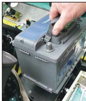
Fig. 10-2 Replacing the battery
