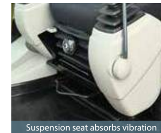
Suspension seat absorbs vibration
