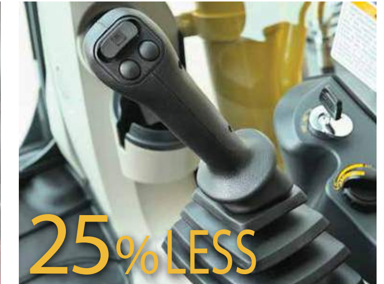
It takes 25% less effort to work the operation lever, which reduces fatigue over long working hours or continuous operations. *Compared to SK170LC-9 model
