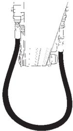
2. Run the hydraulic oil through the carrier's oil filter, for approximately 3 minutes, to make sure that the hoses are clean.
