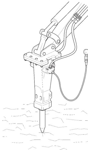
Position the hydraulic breaker vertically towards solid bedrock or similar to adjust the pressure using a pressure gauge.
