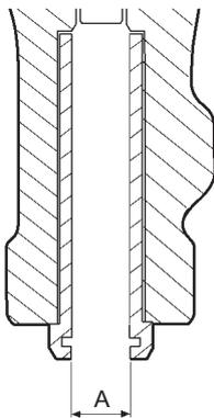
The wear bushing must be replaced when the inner diameter (A) has reached its maximum wear limit, see section "Wear limits" and "Replacing the working tool bushing".
