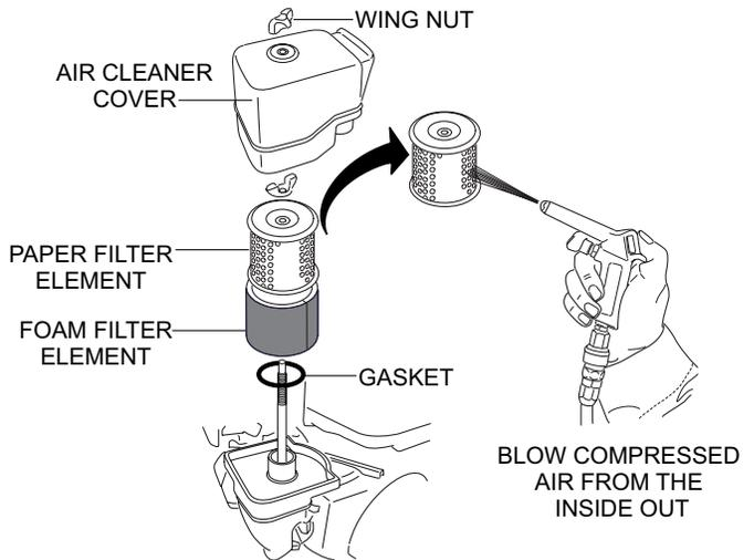
Figure 26. Engine Air Filter (Cyclone Type 2)
