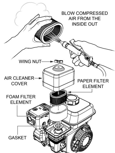
Figure 24. Engine Air Filter (Dual)
