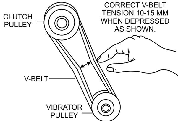
**Figure 10. V-Belt Tension**
