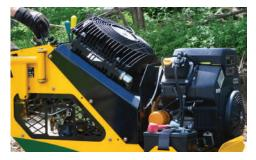
**SET UP FOR STEADY COOLING.** The machine is equipped with a heavy-duty hydraulic oil cooler and reservoir to help manage system temperature increasing reliability and performance.
