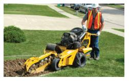
**NARROW WIDTH.** Due to the small size of the machine, it can access small and confined spaces, including maneuvering through typical backyard gates.
