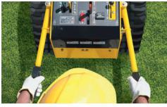
**VZ STEERING.** Instead of additional levers and steerable wheels, operators can turn the machine using only the handlebars. These bars also provide additional leverage when operating in difficult terrain.
