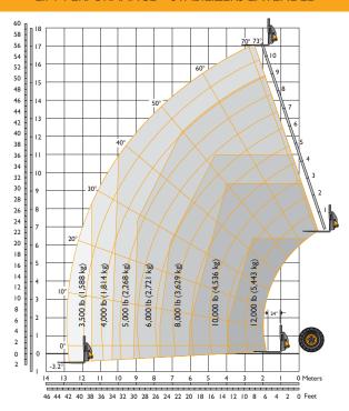
These load charts are for the rated capacity of the machine with 72" wide standard carriage and 48" pallet forks.
