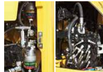
Fuel water separator/Fuel filter/Control valve
