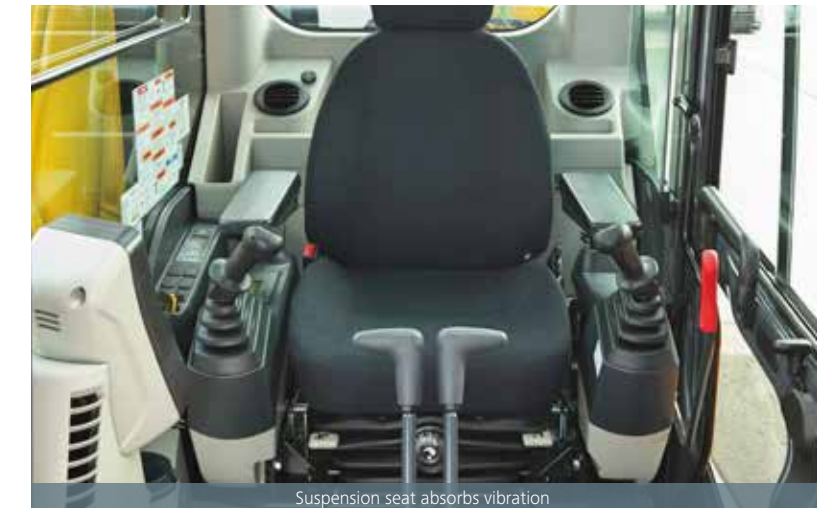
Suspension seat absorbs vibration
