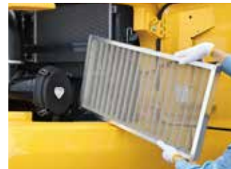
iNDr filter/radiator reservoir tank/air cleaner access.
