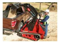
MAXIMUM HEIGHT & REACH 81" hinge pin height allows operator to dump into 30-yard dumpster or side of one-ton truck.
