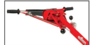
Positive pitch handles use a ratcheting action to provide easy adjustment with the push or pull of a lever.
